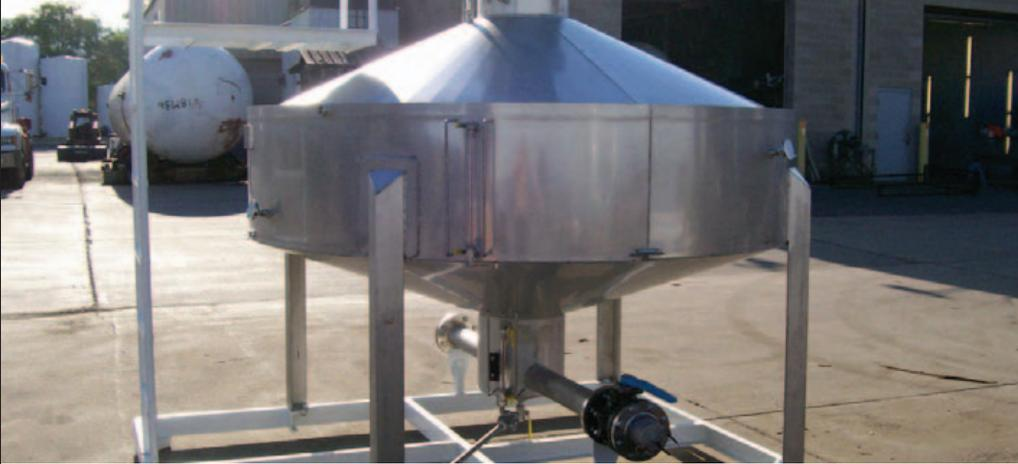
Tank Provers of varying sizes for 4" Volumetric Meters
